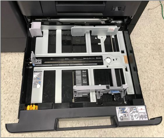
Both length and width guides slide in sync when adjusting paper size in the drawers and have blue locking tabs for easy view. The drawers also feature easy-to-see limit indicators for standard paper, envelopes, and small sizes. The soft close drawers make for no slamming of cassettes, and also pull out far enough for easy access in case of misfeed.
