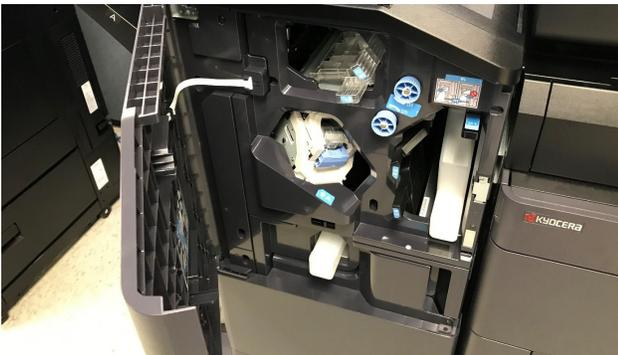
Misfeed areas are easily identified inside the machine with blue labels and numbers.
